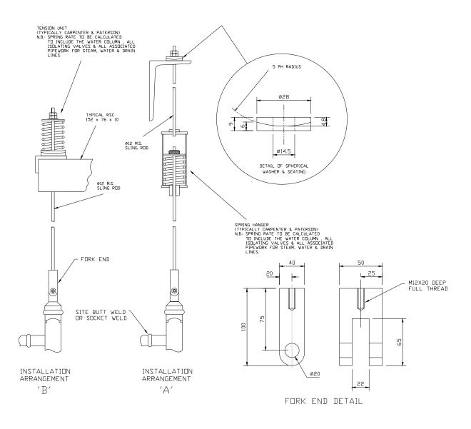
Figure 2.3 - Typical water column suspension
